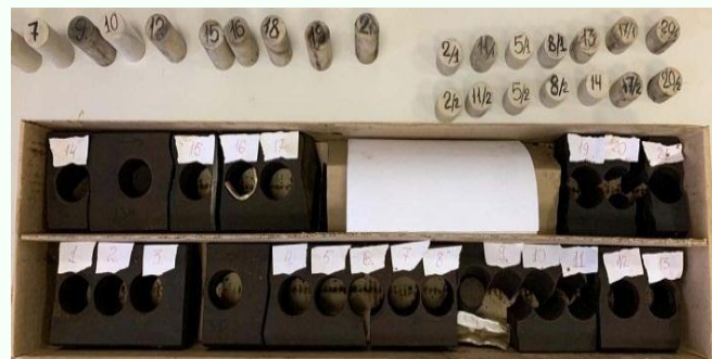
Fig.1. Source core material and samples after drilling out
