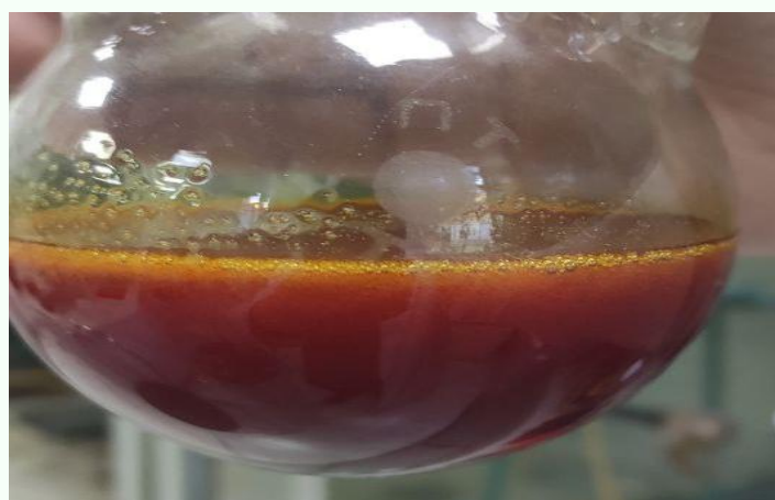
Figure 2. Alcoholysis product synthesized at 190°C for 6 hours.
