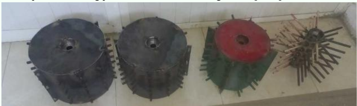
Figure 3.2. Improved pile drum
